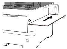
When the paper is inserted all the way in, stapling takes place.
