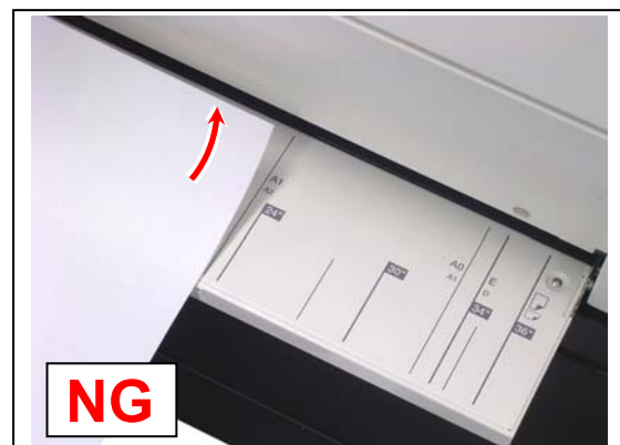
Incorrect (curl up)
