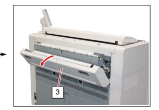
5. Pull and remove the jammed print to the rear.
