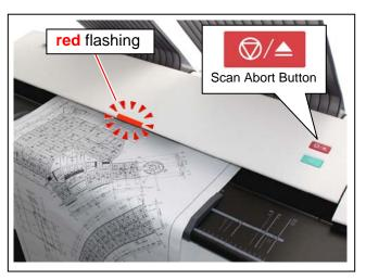
Pressing the button stops the current reading a document immediately. The current printing is stopped as well and is ejected.
