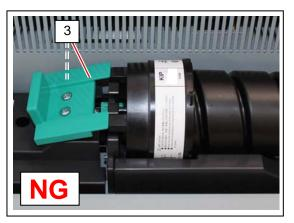
7. Turn the body (4) of the cartridge in two or more revolution to the arrow direction to open the toner supply hole. Confirm that the projection (8) if fitted into the notch (9).
