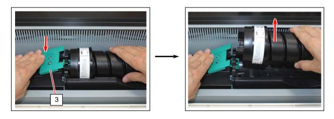
5. Shake the new Toner Cartridge left and right 5 times or more to make the toner smooth. After shaking, tilt the Toner Cartridge to the cap side.
