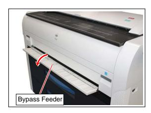
2. There are several size markings on the table of Bypass Feeder which indicate possible feed positions. Place the cut sheet paper on the table between its concerning size markings then insert it into the Bypass Feeder.
