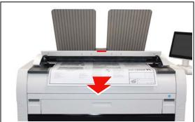
2. Gently press Scanner Unit down and firmly close it.
