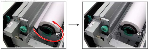
3. Insert the leading edge of the roll media under Guide Plate (2) until it touches the feeding roller. Rotate Feed Knob (3) clockwise so that the feeding rollers catch the leading edge.
