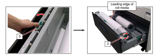
5. Slide the green Cutter Knob (6) fully from one side to the other to make a new straight edge. Remove the cut portion.
