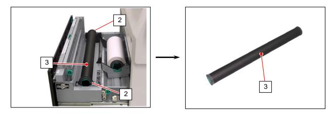
3. Raise the green lever (4) on Flange (2). Remove both Flanges (4) from the roll core (3).
