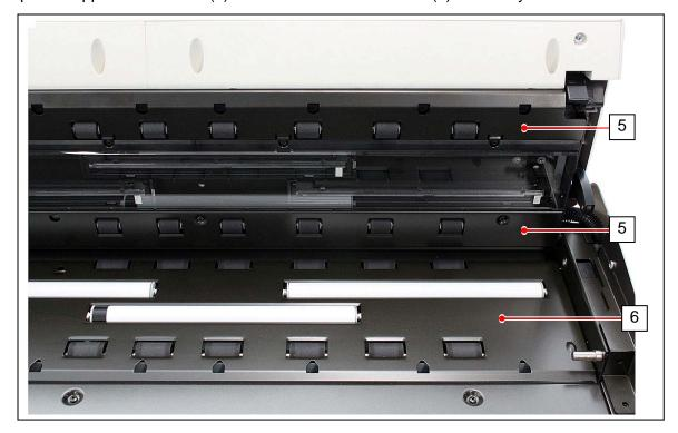
7. Gently press Scanner Unit down and firmly close it.
