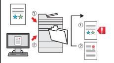
When paper empty error occurs at the cassette by specifying the special paper size or type, the machine skips the error job and perform the next job.
