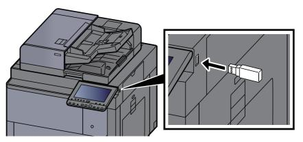
When the machine reads the USB memory, "Removable Memory is recognized. Displaying files. Are you sure?" may appear. Select [Yes].
