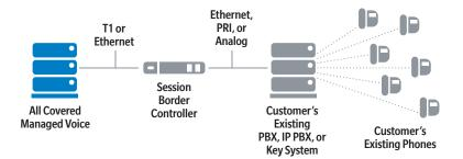
Utilizing the client's existing internet connection, SIP Trunking provides a blend of voice and data traffic onto a single IP circuit. This service delivers dynamic bandwidth allocation while supporting FXS, PRI, and T1 connections. The benefits include one network connection, one bill and one point of contact for local, long distance and simplifying the overall experience.
