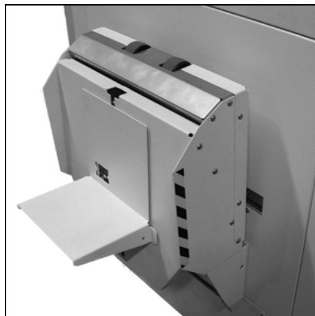
FIGURE 31. The stacker in raised position
