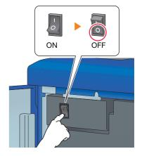
$11 \quad \text{Turn the power switch in the rear side off.}$
