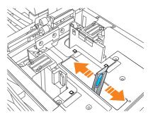
5 To fix the **side guide plates** at the correct locations, load an appropriate amount of paper into the tray while aligning it to the left-hand side of the tray.
