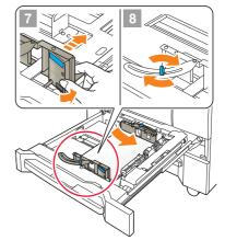
9 Load the remaining paper into the tray, then press the rear guide plate against the paper.
