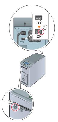
→ For Image Controller IC-314, open the front door and press the Power controller button.
