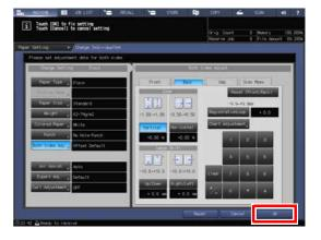
19 Press [Close] to exit the adjustment. Chart Adjustment is then completed.
