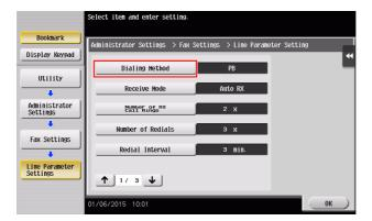
For the push-button type, select [PB], and for the dial-pulse type, select [10pps].
