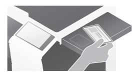
If biometric authentication is enabled, put your finger on the finger vein reader of the authentication unit.
