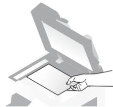
Load the original face up into the reverse automatic document feeder.
