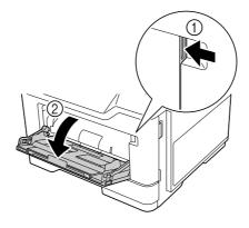
2 Pull out the extension guide of the **Bypass Tray**.
