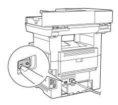
The **Start** key lights up orange, and a screen appears to show that this machine is in the process of start-up.
