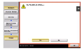
12 Make sure that a message appears prompting you to turn OFF and then ON the **main power switch**. Now, turn OFF and then turn ON the **main power switch**.
