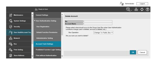
→ If the boxes are changed to Public User Boxes and if the password set for a particular box before this change does not meet the Password Rules, no access can be made to the Public User Box, to which that specific box was changed. In this case, the administrator must first newly set a password that meets the Password Rules. For details of the Password Rules, see page 1-13.
