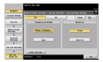
→ Under [Overwrite], whether to enable writing over old Job Logs when the Job Log space in the HDD is full of old Job Logs can be selected.
