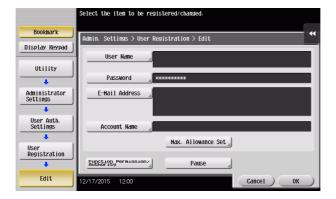
→ If Account Name is not registered, Account Track becomes necessary even with [Synchronize] set for [Synchronize User Authentication & Account Track]. Account Track is, however, necessary only for the first time. Once any account is authenticated, that particular account is registered for Account Name. The machine can thereafter be used only through User Authentication.
