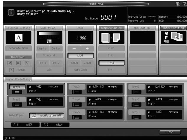
7 Measure the misalignment between front and back sides using the points ([a] to [d]) on the [back] side of the chart to determine the adjustment value.
