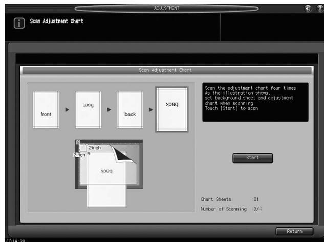
→ When four times of scanning are completed, a dialog is displayed to calculate the adjustment value.
