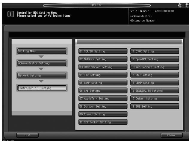
Selecting [ON] for the IWS (Internal Web Server) Setting enables you to have a print data conversion application transferred to this machine and to utilize the print data conversion function. Contact your service representative, if desired.
