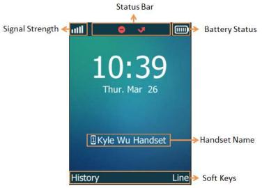
The LCD screen is divided into three parts: Status Line, Text Line and Softkey Line.
