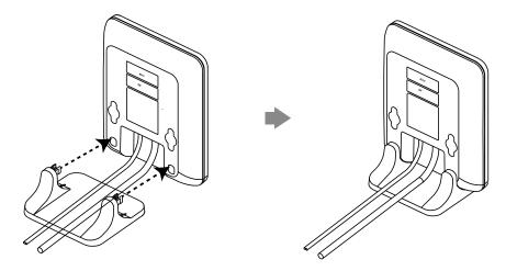
Align the snap-fits with the corresponding holes and push forward, snapping them into the holes.
